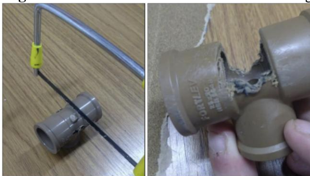
Figure 4: Hole for thumb control of tube sliding
