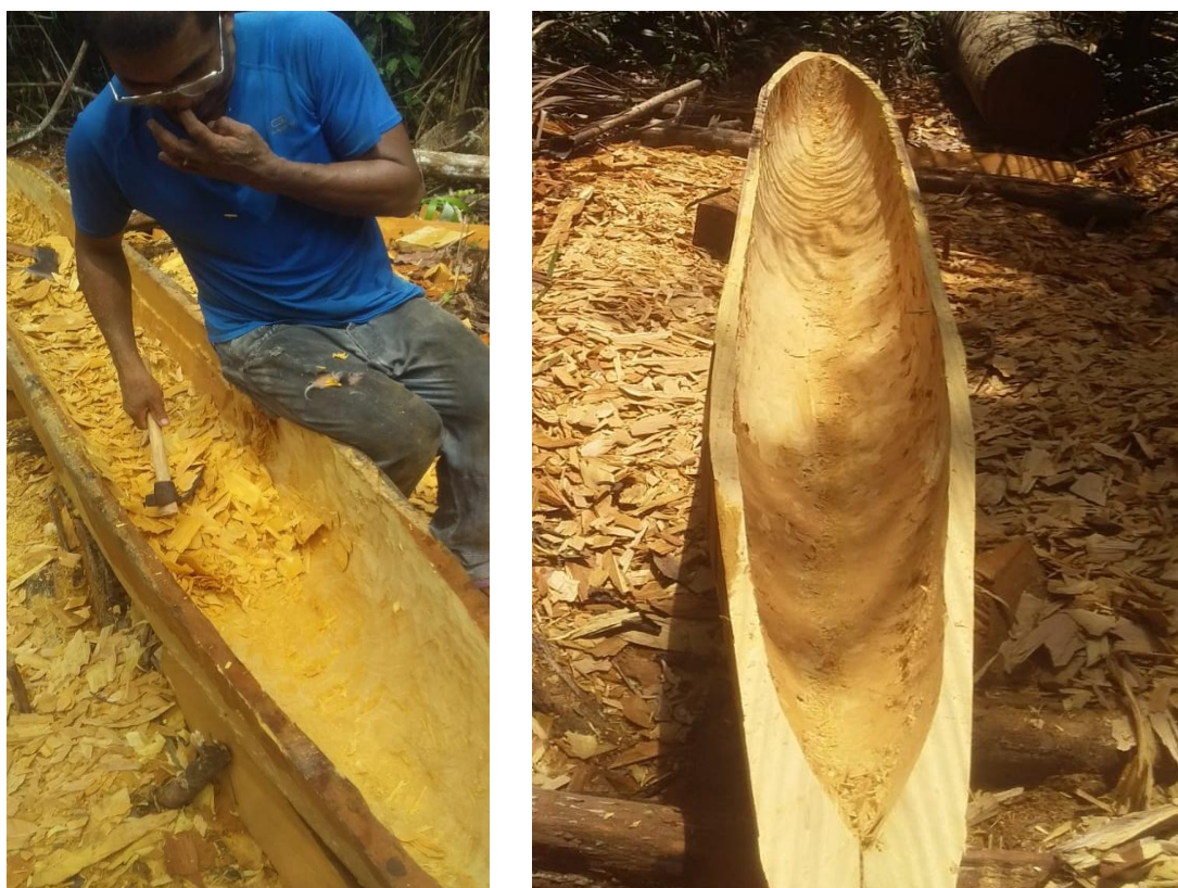
Figure 05: Cleaning the hull opening
