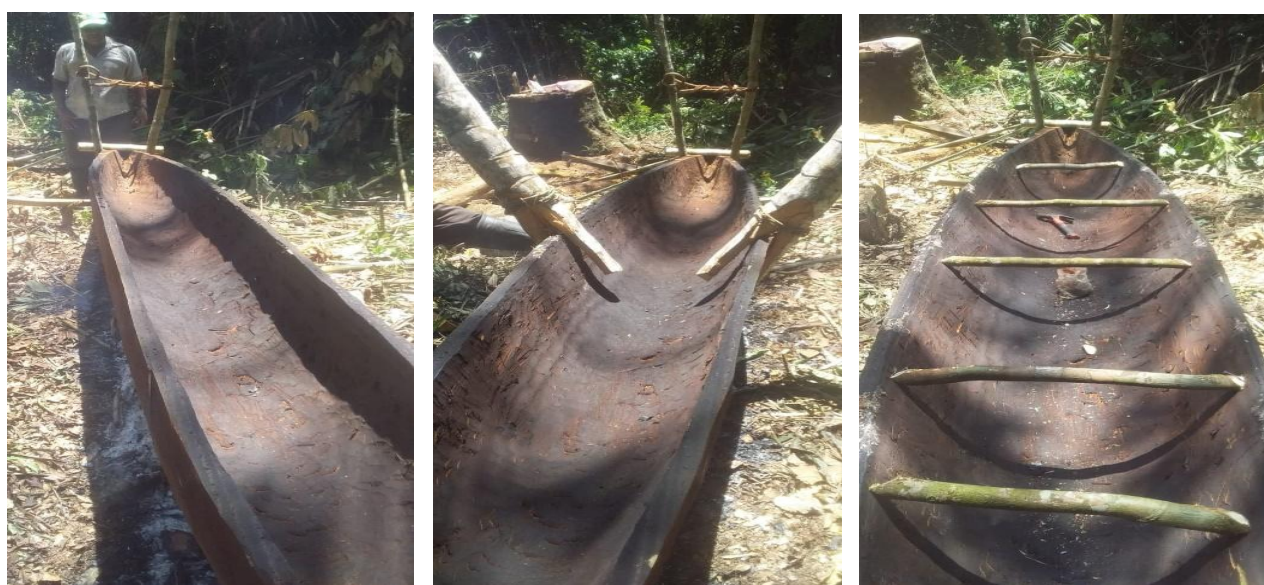
Figure 07: Hull opening (final process)
