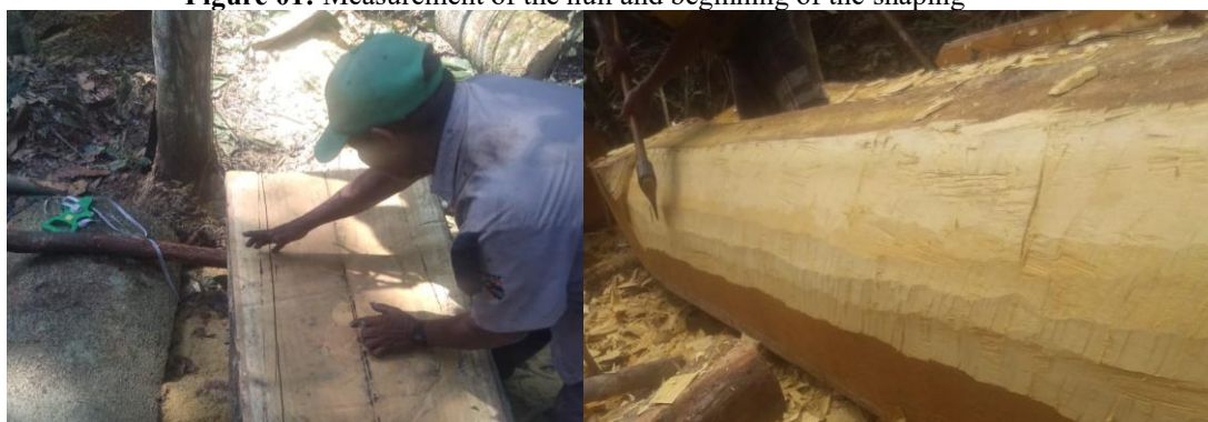
Figure 01: Measurement of the hull and beginning of the shaping
