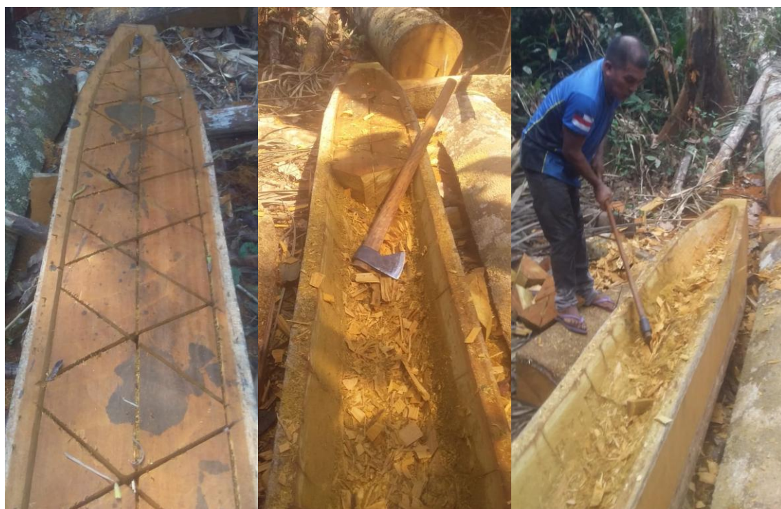
Figure 04: Some steps of the hull excavation
