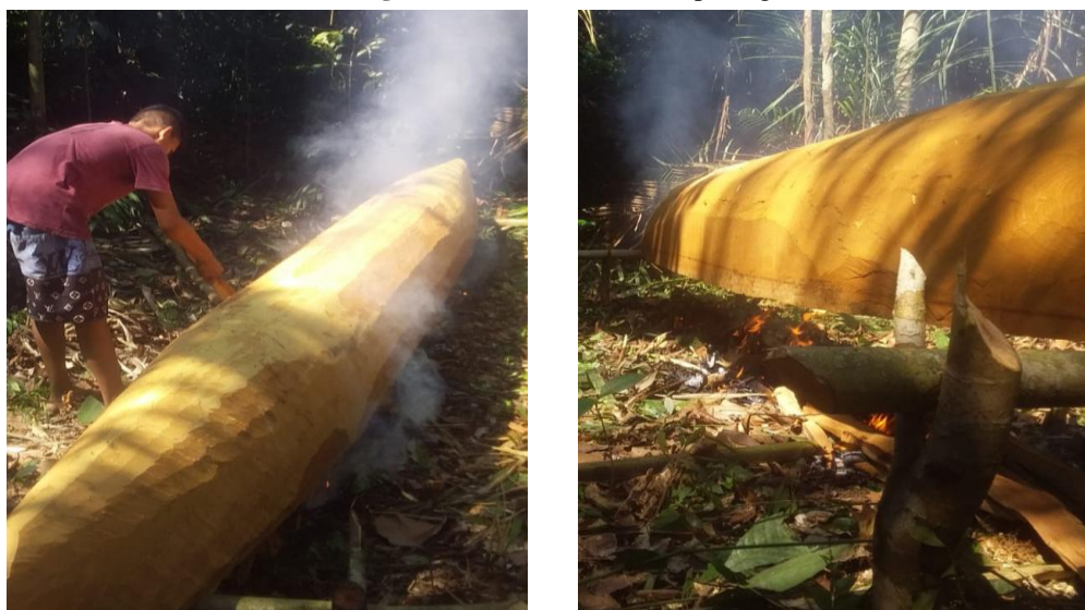
Figure 06: Fire for the hull opening
